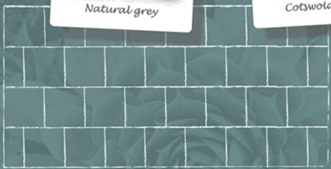
Staggered joint using 450 x 450mm slab
